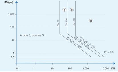
DN x PS > 1000 : Gas / liquid = compressed air DN = inner diameter PS = maximum pressure
