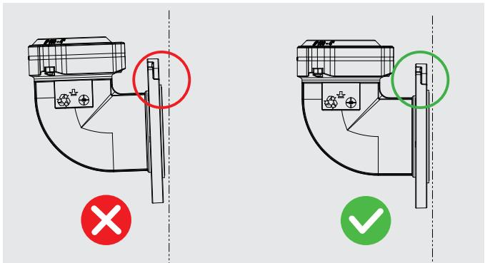
**! WARNING:** Check alignment before tightening for a secure connection.
