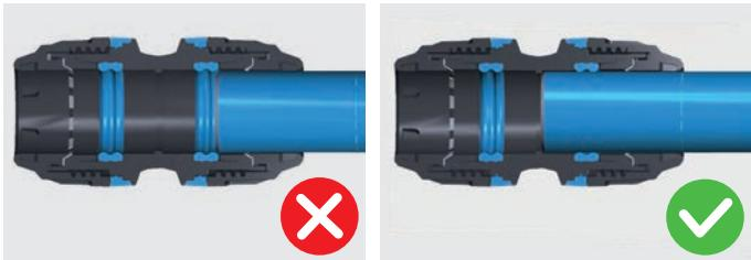
3. Check the presence and positioning of all components in the fitting.
