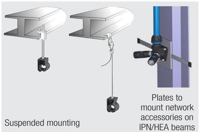
To guarantee the system is aligned and solidly attached, select an appropriate mounting option depending on the configuration of the building. For safety purposes, we recommended mounting clamps no more than 3 m (9 ft.) apart.
