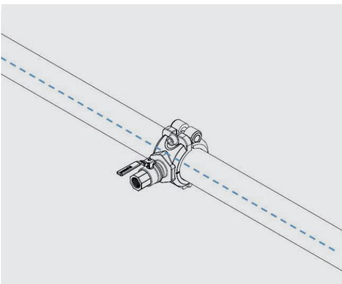
Use the notches as a guide to mark the position on the pipe with a felt tip marker.
