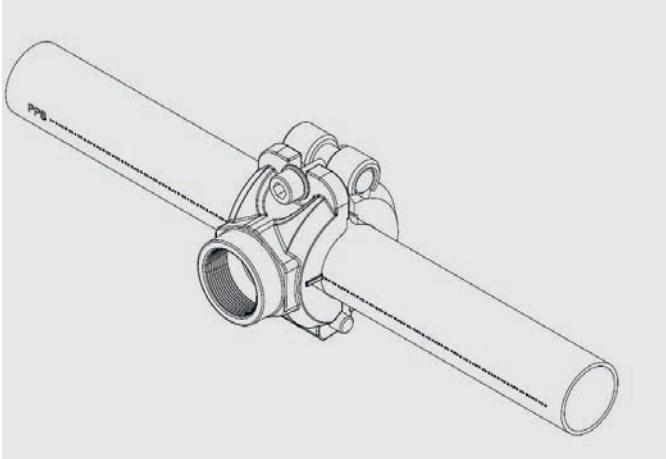
Use the notches on each side of the tapping flange to set the fitting to its desired position on the pipe.
