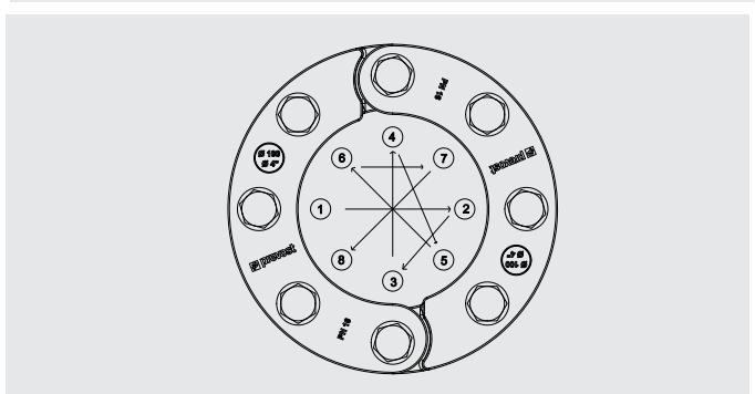
Repeat this step 2 or 3 times, until tightening torque 30 Nm is reached.
