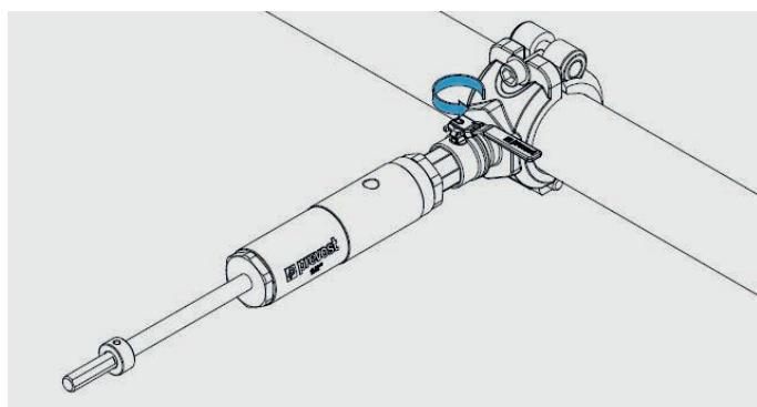
Unscrew the drilling tool **PPS DRIL**.
