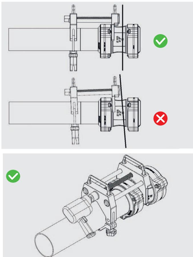
For a secure fit, all parts of the fitting must be aligned on the pipe.
