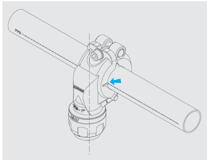
Use the notches on each side of the tapping flange to set the fitting to its desired position on the pipe.
