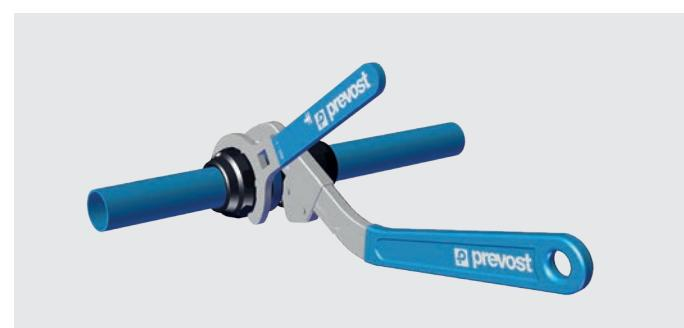
Use the **PPS1 CLESTD** (neutral hook spanner) to hold the body of the fitting in position while using the **PPS1 CLE** wrench to tighten the nuts.
