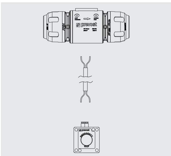
Connect the pneumatic valve to the remote pilot using 2, Ø 0.15" PA tubes. Note the "PILOT PRESSURE" and "CLOSING PORT" areas on the unit.
