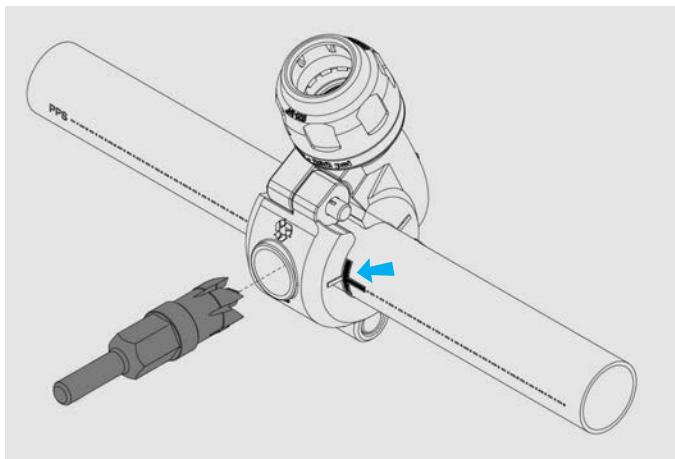
**Warning:** The pipe must be deburred before using this tool.
