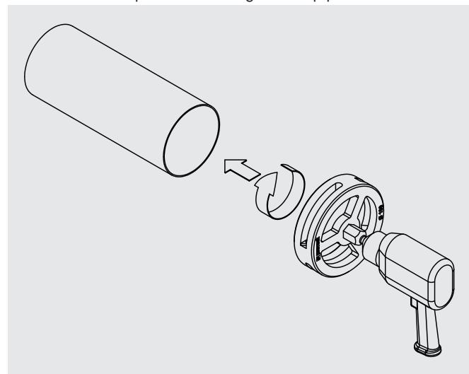
Do not exert excessive pressure on the pipe.
