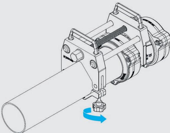
**⚠ WARNING:** Check for proper alignment of the pipe and the fitting to avoid leaks prior to tightening the nut.
