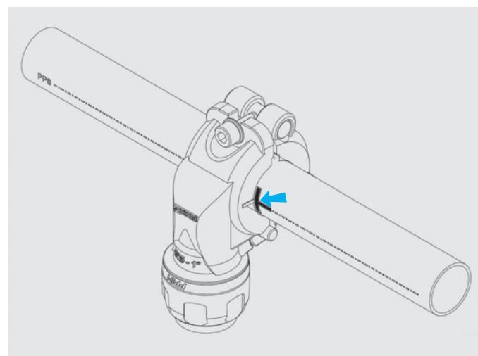
Use the notches as a guide to mark the position on the pipe with a felt tip marker.
