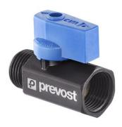
NPT male thread NPT female thread **Technology** Operating pressure 1/2" MNPT 1/2" FNPT PPS Grip Concept 0 to 232 psi Construction Vacuum capability Highlight Temperature -4°F to +176°F Pipe and fittings: aluminum Scalable system -29 inHg (vacuum 98%) Meets standards ASME B31.3 REACH
